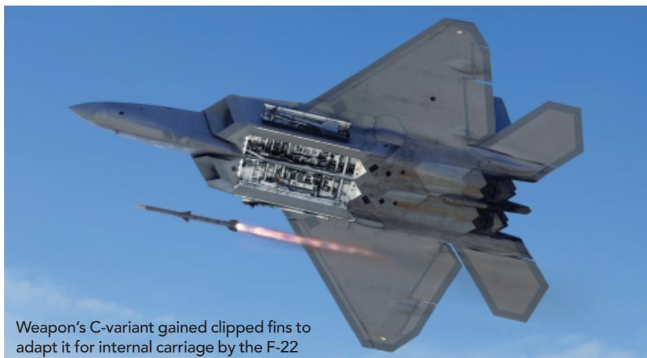
Weapon’s C-variant gained clipped fins to adapt it for internal carriage by the F-22
