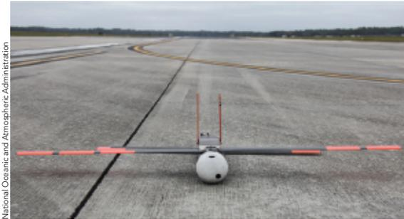
Tube-launched air vehicle weighs just 5.9kg
