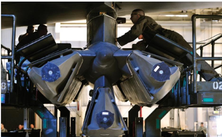
Aged B-52H can carry multiple AGM-86B air-launched cruise missiles on underwing pylons
