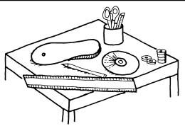
1. You need an old rubber slipper, discarded CD, 6 ring magnets (17.5-mm OD, 7.5-mm ID, 3-mm thick - they cost 1 rupee each), one pencil and few simple hand tools.
