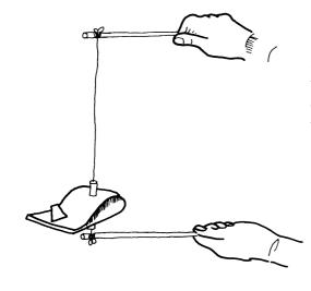
3. Stick a piece of paper on the centre line of the trailing edge. This fin will stand vertically on the trailing edge and will help in stabilising the wing. Pass a thin thread through the refill and fix it on two sticks.
