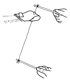
4. As you swing the sticks through the air the wing will rise on the thread. The top curved portion of the wing is longer than the bottom portion, so the air moving over the top has further to go and therefore it moves faster. This produces a lower pressure on top of the wing producing lift. This is how a wing helps an aeroplane to rise in the air.
