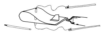
2. Make a hole straight through both parts of the wing about 3 cm from the leading edge. Pass a piece of empty ball pen refill or soda straw through it and fix it with a dab of glue.
