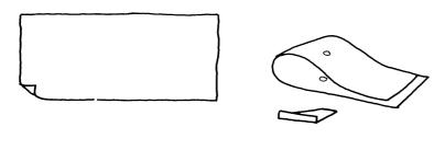
1. Cut a piece of paper 20 cm long and 10 cm wide. Bend it in half as in and stick the edges together. Run a fold along the edge with your finger nails so that it bends, curved at the top and almost flat underneath. The flat end of the wing is the leading edge, and the thin edge is the trailing edge.
