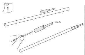
Remove the brass tip of an old ball pen refill. Push the ball out of the tip with a needle. Now the tip will have a jet like orifice.
