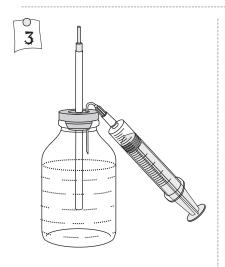
Fill the glass bottle with water and then fix its lid. Also bend and push the needle of a NEW syringe in the lid.
