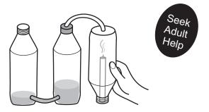
6 After a while the candle will consume all the oxygen in the bottle and will extinguish. A partial vacuum will be created and some water will be sucked into the middle bottle. The level of water in the middle bottle will rise.
