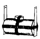
12. The metal strips serve three purposes. They act as power leads, supplying current to the coil. They are also bearing supports for the coil. Finally, they also make a stand for the motor.
