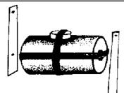
11. Stretch out another cycle tube rubber band (1-cm wide) along the length of the battery. Now insert the stove pins in the rubber band. The pin with two holes is placed next to the flat end of the battery. The second hole bites into the plane end of the battery and makes a good electrical contact.
