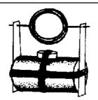
13. Now pull the metal strips a little apart and slip the motor coil in their holes.
