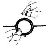
4. Tie the coil at several places with little bits of string. The string will keep the loops of the coil in place.
