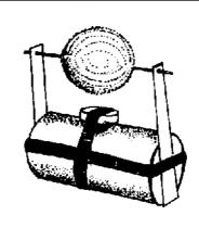
14. Give the coil a gentle starting push and it will start rotating. However, if the push is in the wrong direction, then the coil will stop after a while, flip, and rotate in the right direction.
