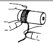
2. Take 1-metre of Copper wire (20 gauge). Straighten it by running it through a piece of cloth . Wind it tightly on a torch battery. The loops of the wire should be adjacent to one another. They should not overlap. The coil should have about 10 turns.
