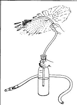
5. Water will keep sprinkling out as long as you continue spinning the tube. This way you can drain out the whole bottle. The centrifugal force of rotation is enough to suck and lift water from a height of almost a metre. You can make a simple foot valve using a cycle steel ball and a pen body as a seat.
