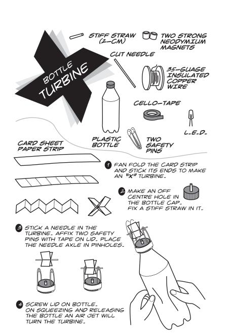
NOW CUT THE BASE OF THE BOTTLE AND MOVE IT UP AND DOWN IN A JAR OF WATER. AIR EXPELLED FROM THE BOTTLE WILL CONTINOUSLY TURN THE TURBINE.
