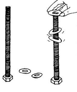
1. Take an 8-10mm diameter 20 cm long steel bolt. It will be very nice if you can get a long stud. Also get a few steel washers slightly larger than the diameter of the bolt. Stand the bolt vertically and place the washers on top. The washers will go down the bolt in a very funny "dancing" fall. For the most spectacular result you'll have to try a few different sizes of washers.
