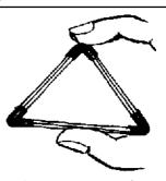
9. But no matter how hard you press, a triangle remains a triangle. The triangle is the only rigid polygon. That is why roof trusses, bridges, electricity towers are made of triangles. The triangles make them rigid and strong.
